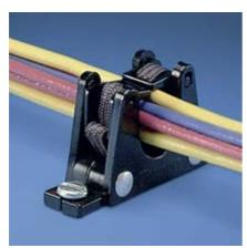
ER Type retainers form wire bundles as wires are inserted. Completed bundles then snap out. Two sizes available for 1/2" (12.7mm) and 1 1/4" (31.7mm).
