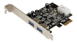
The PEXUSB3S25 2-Port PCI Express USB 3.0 Card lets you add two USB 3.0 ports to your PCI Express-enabled computer system, with an optional LP4 power connector to connect to your system power supply and deliver up to 900mA of power per port to USB 3.0 bus-powered devices (500mA for USB 2.0).
