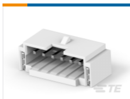
TE Part # 2381626-6 1.5P 6POS WTB R/A BRD W LATCH TIN NAT
