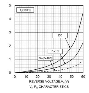
REVERSE POWER DISSIPATION:P<sub>R</sub>(W)
