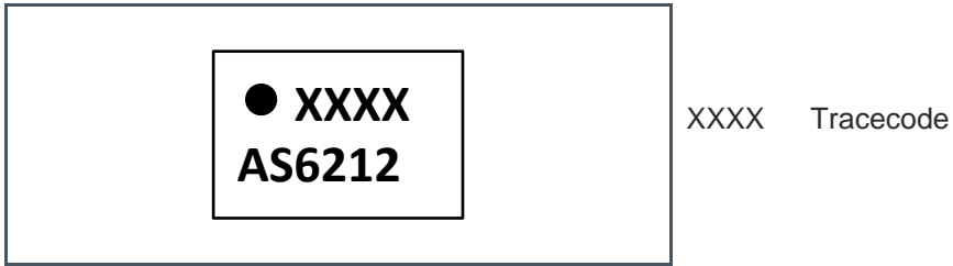
Figure 38: WLCSP Package Marking/Code for AS6212
