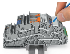
Inserting a conductor via push-in termination. Solid conductors with cross-sections from either one size above, or up to two sizes below, the rated cross-section can be simply pushed in – no tools needed.
