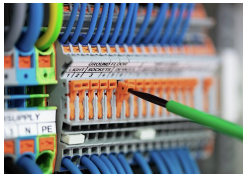
Pivoting a knife disconnect.
