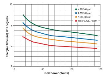
Graph 2 shows operation end-to-end. Note the high starting torque for high starting acceleration or for stopping the load by means of reverse voltage at the end of the stroke. If the device is used in a full stroke application, the load can be externally latched, detented, or biased to either end of stroke.
