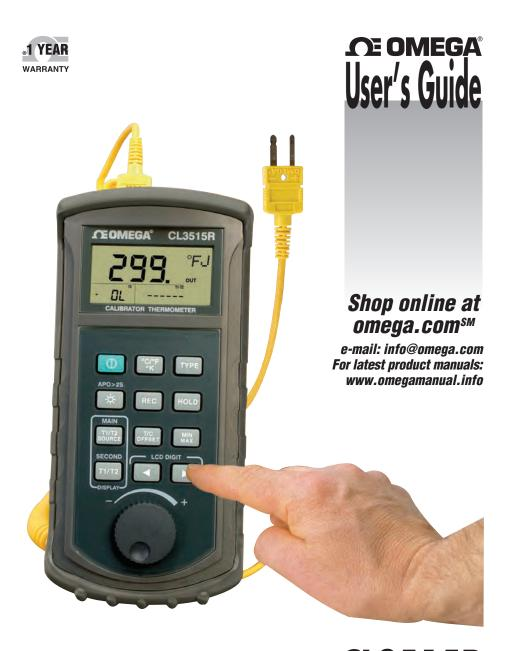
CL3515R K/J/T/E/R/S/N/L/U/B/C Calibrator Thermometer
