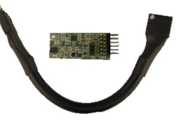
the Multi-sensor board, is an ideal choice for mobile applications that need ambient light sensing. The inertial sensing on the board is provided by Bosch's BNO055, a 9axis absolute orientation sensor that includes an accelerometer, gyroscope and a magnetometer. BME680, from Bosch provides gas, pressure, humidity and temperature sensing capabilities on the Multi-sensor board.
