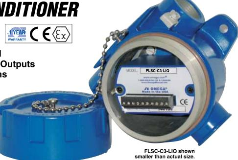
The FLSC-C3-LIQ is a DC powered, microprocessor controlled transmitter. It outputs a pulse scaled per unit of flow, and analog signal proportional to flow rate.
