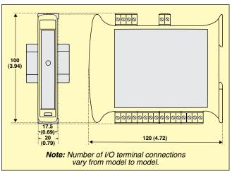
Dimensions: 17.5 W x 100 H x 120 mm D (0.69 x 3.94 x 4.72") Weight: 150 g (6 oz); 210 g (8.4 oz) HE359DIQ512 only Communications: MODBUS®/RTU (binary) RS485 half duplex Default Communications Parameters: 38400 baud, N, 8, 1, no h/s default modbus ID 1 Supported MODBUS Commands:
