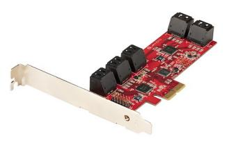
This 10-port SATA III (6Gbps) controller enables you to add 10 SATA 6Gbps Hard Drives (HDDs) or Solid State Drives (SSDs) to your computer system or server via an available PCIe x2 card slot. The card supports SATA III and PCI-Express 2.0 Specifications.
