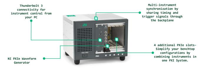
With the PXI waveform generators, generate standard functions and user-defined, arbitrary waveforms as part of a PXI system. The PXI Waveform Generator bundles feature up to 2 output channels with up to 80 MHz bandwidth,  $\pm$  12 V output range and 800 MS/s maximum update rate.
