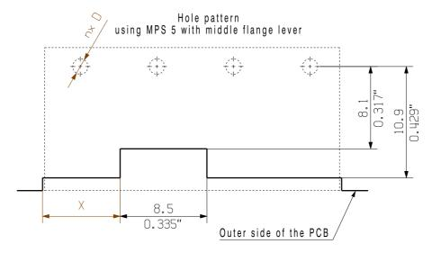
Hole pattern Using MPS 5 with middle flange lever
