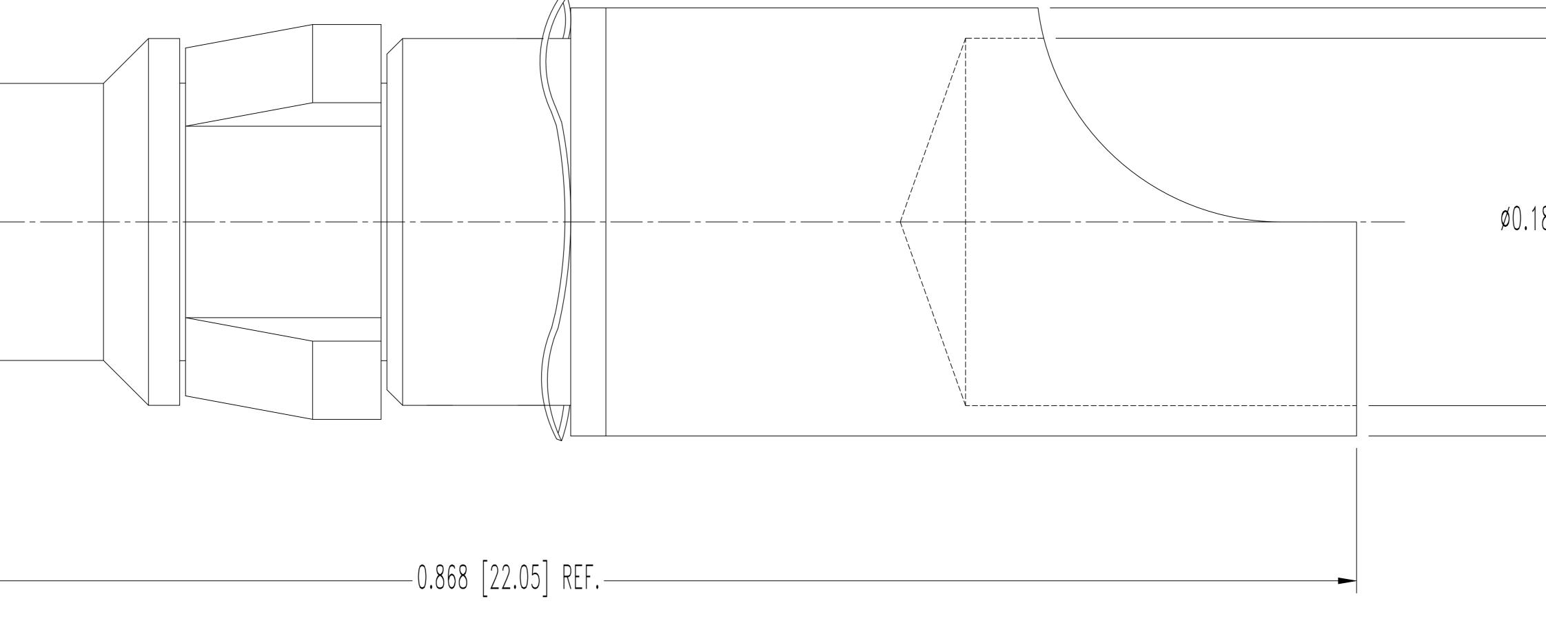
1. MATERIAL AND FINISH: HIGH CONDUCTIVITY COPPER ALLOY, 0.000030 [0.75µ] GOLD OVER NICKEL OVER COPPER.
