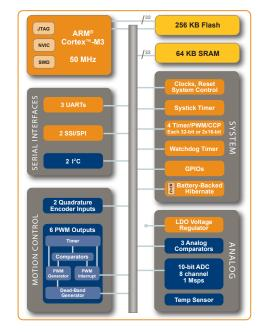
**LM3S2000 Series Block Diagram.** This block diagram shows the superset of features for the LM3S2000 series of microcontrollers.
