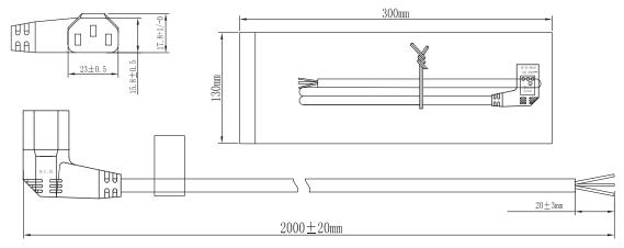
CABLE MARKING: H05VV-F 3G0.75mm<sup>2</sup> ⊲ VDE ⊳ N19626 CCC A030116 No.2003010105097406 227 IEC 53 (RVV) 300/500V 3X0.75mm<sup>2</sup>
