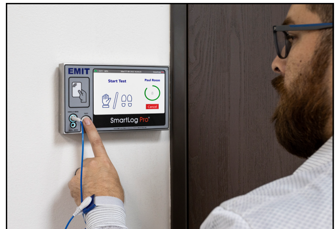
Figure 24. Performing a single-wire wrist strap test
