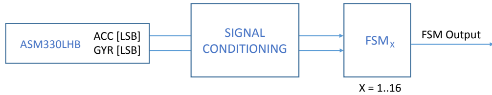
Figure 2. State machine in the ASM330LHB
