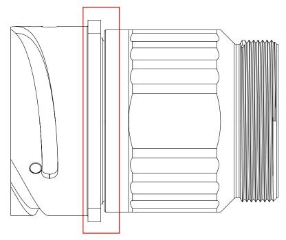
The recommended installation torque for the part in the red box as shown in the Figure is 160~170 Lbs. (The Plug connector is the same as the Receptacle Connector)
