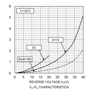
REVERSE POWER DISSIPATION:P<sub>R</sub>(W)
