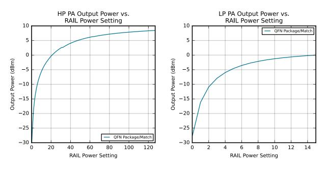
Figure 4.12. Transmitter Output Power, QFN Package / Matching
