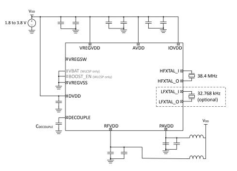
Figure 5.1. Typical Application Circuit: Direct Supply Configuration without DCDC (EFR32xG27C1x or EFR32xG27C3x)
