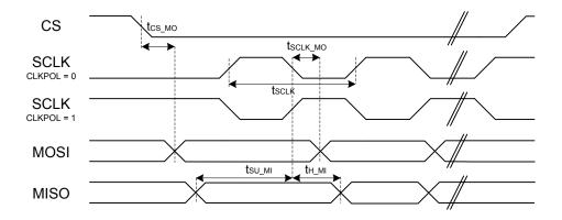
Figure 4.5. SPI Main Timing (SMSDELAY = 1)
