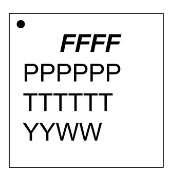
Figure 7.3. QFN32 Package Marking
