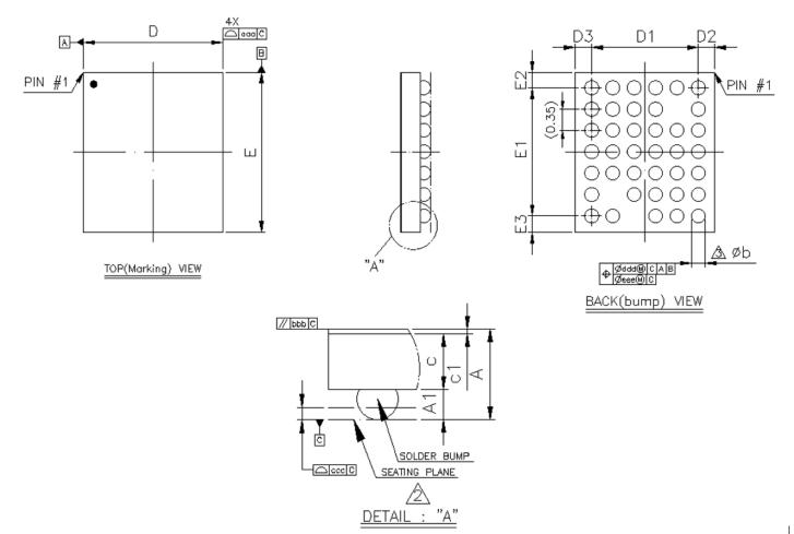
Figure 9.1. WLCSP39 Package Drawing
