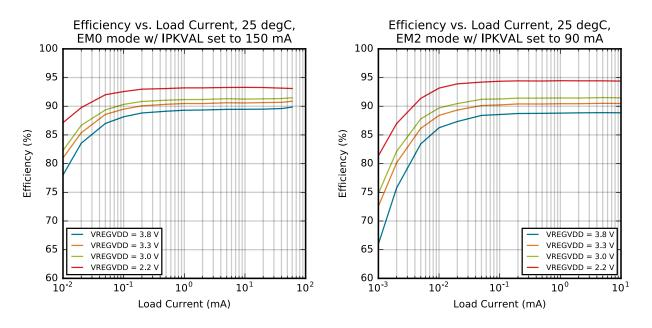
Figure 4.14. Buck DC-DC Efficiency
