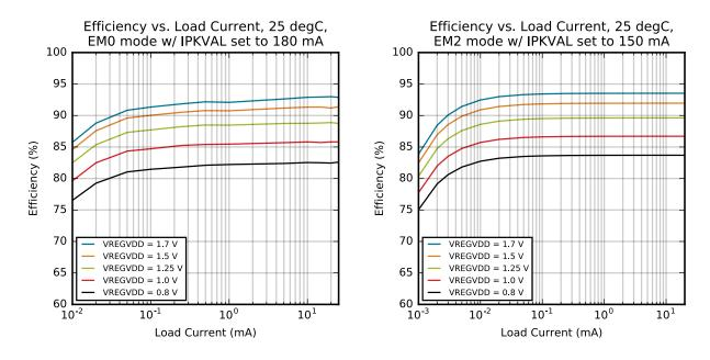
Figure 4.15. Boost DC-DC Efficiency
