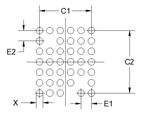
Figure 9.2. WLCSP39 PCB Land Pattern Drawing
