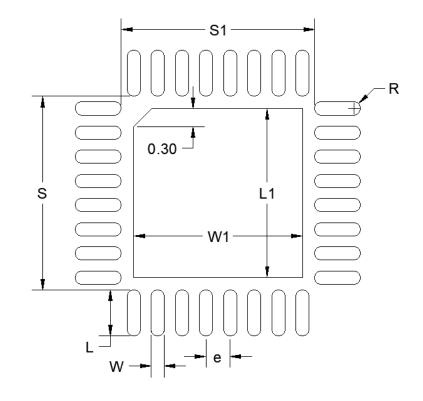
Figure 7.2. QFN32 PCB Land Pattern Drawing
