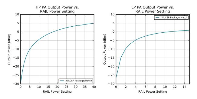
Figure 4.13. Transmitter Output Power, WLCSP Package / Matching
