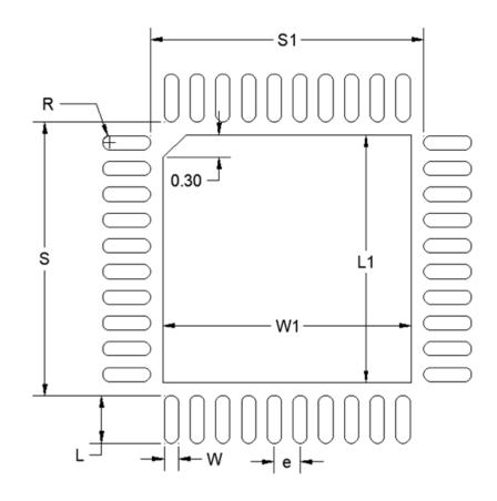
Figure 8.2. QFN40 PCB Land Pattern Drawing
