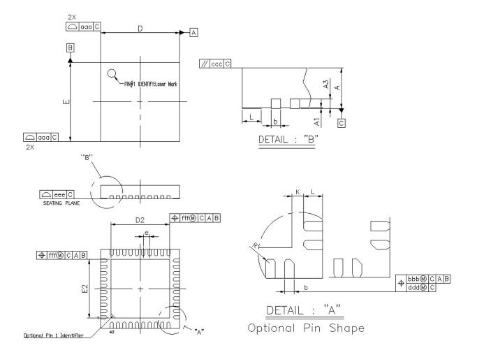
Figure 8.1. QFN40 Package Drawing
