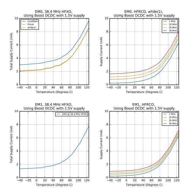
Figure 4.10. EM0 and EM1 Typical Supply Current vs. Temperature (Boost DCDC)
