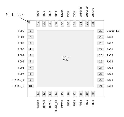
Figure 6.1. QFN40 with Buck DC-DC Device Pinout
