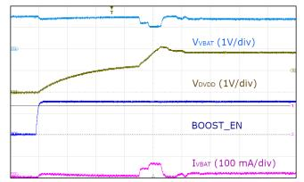
Time scale = 1 ms / division  $V_{VBAT}$  = Input voltage at pin, 1.5 V source with 10 Ohm impedance  $V_{DVDD}$  = Output voltage at pin, target 1.8 V BOOST\_EN = Boost enable input pin  $I_{VBAT}$  = Current seen at VBAT input pin
