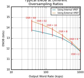
Figure 4.17. Typical ENOB vs. Oversampling Ratio
