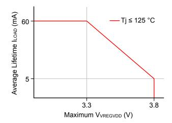
Figure 4.1. Lifetime average load current limit vs. Maximum input voltage
