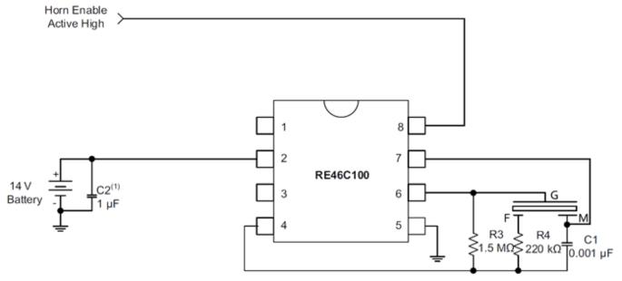
Note 1: Place C2 close to the device power pins to minimize horn switching noise.
