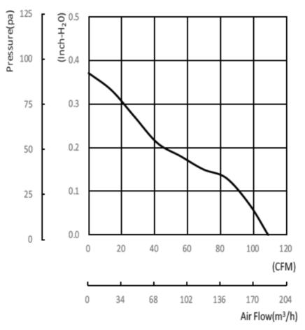
**Air Flow & Static Pressure Curve**
