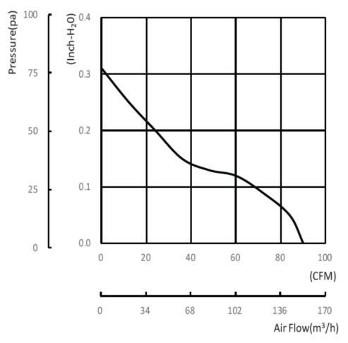
**Air Flow & Static Pressure Curve**
