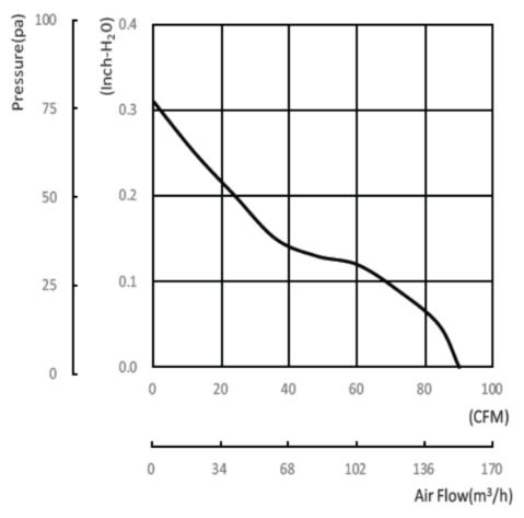
**Air Flow & Static Pressure Curve**
