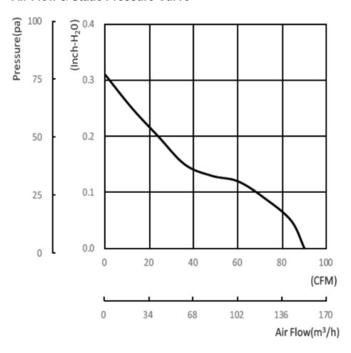
**NOTE**: The airflow and static pressure are measured with specific fixture.
