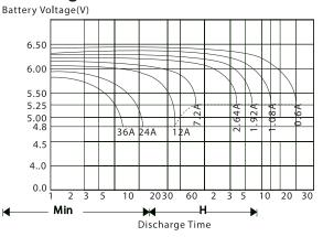
Note:Discharge shall be cut-off at 5.25V if discharge at 1CA and at 9.6V if at  $\ge$ 1CA
