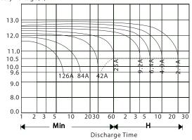
Note:Discharge shall be cut-off at 10.5V if discharge at 1C<sub>A</sub> and at 9.6V if at  $\geq$ 1C<sub>A</sub>
