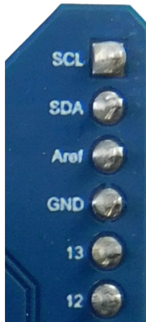
Figure 3. CN2 connector for I 2 C/I 3 C connection
