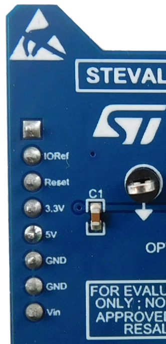
Figure 2. CN1 connector for 3.3V power supply
