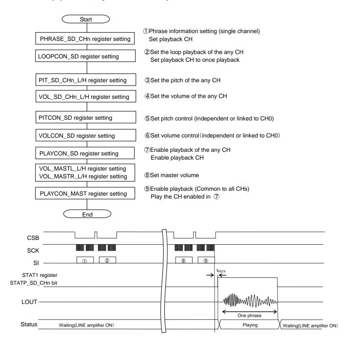
SoundGenerator can select once playback or loop playback depending on the presence or absence of loop setting. When playing once, the playback ends at the same time as the phrase ends.
