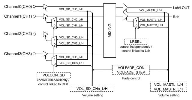
The combination of volume control for each channel is as follows.
