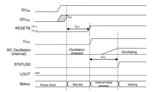
When turning on the power, enter "L" in the RESETB pin.
