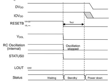
When turning off the power, enter "L" in the RESETB pin.
