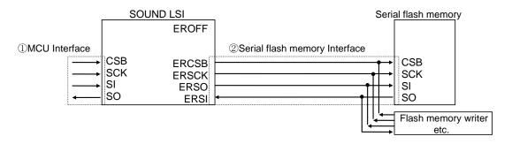
① Rewrite using the clock synchronous serial interface of the MCU interface
