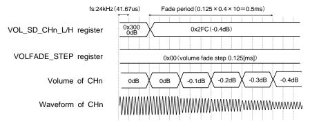
The volume transitions according to the sampling frequency (fs). If sound code data of different fs is being played at the same time, the volume transition time will be different. For the volume transition time, refer "VOLFADE\_STEP register" in the "Registers" chapter.
