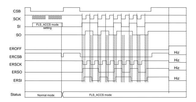
When FLS\_ACCS mode is set, the pins are directly connected inside the LSI as shown below. When the EROFF pin is set to H level, the ERCSB, ERSCK, ERSO and ERSI pins are in the HiZ(high-impedance) state.
