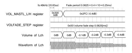
The volume transitions at 48kHz or 32kHz depending on the GFS bit of the OUTMODE register. For the volume transition time, refer "VOLFADE\_STEP register" in the "Registers" chapter.
