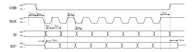
◆ Clock Synchronous Serial Interface Timing (SCK Initial Value = "L" Level)
