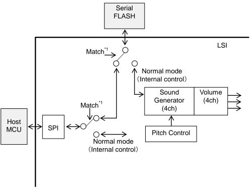
\*1: The write conditions to the flash memory access control register match
