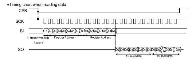
In the two-times input mode, if two-times input error is detected when reading a register, read data "1" is output.
