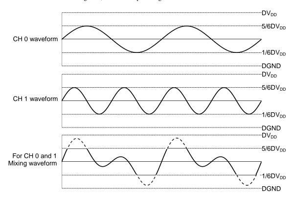
If the result of mixing CH 0 and 1 exceeds from the  $1/6{\rm DV_{DD}}$  to  $5/6{\rm DV_{DD}}$  level (as indicated by the broken line), the sound quality may be reduced by clamping.
