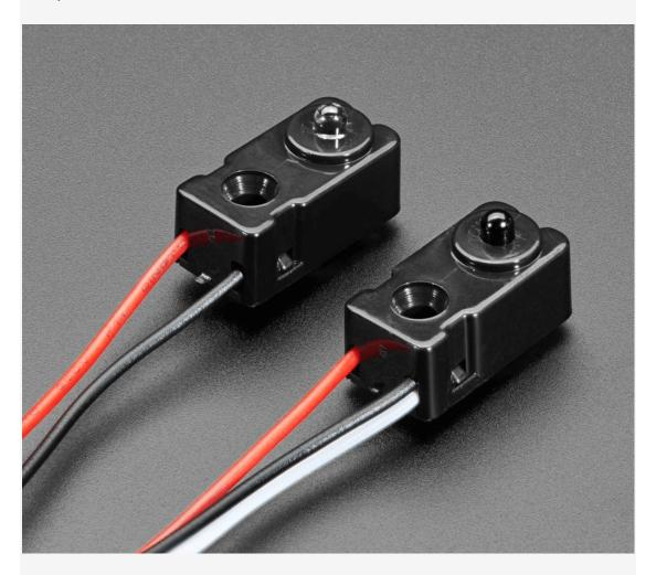
They work by having an emitter side that sends out a beam of human-invisible IR light, then a receiver across the way which is sensitive to that same light. When something passes between the two, and it's not transparent to IR, then the beam is broken and the receiver will output a signal to let you know.
