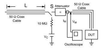
Figure 11. Simplified Schematic of a Typical TLP System
