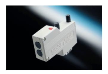
Profibus is the most widely used field bus. It is promoted by Siemens and by organized, interested and committed manufacturers and users in the PNO (Profibus user organization). The IP 20 interface on the device side is standardized as a 9-pin Sub-D female connector. The max. data transmission rate is 12 Mbit/s. The cable is a shielded twisted pair conductor. The cable sheath is violet and the signal cores are green (A) and red (B).
