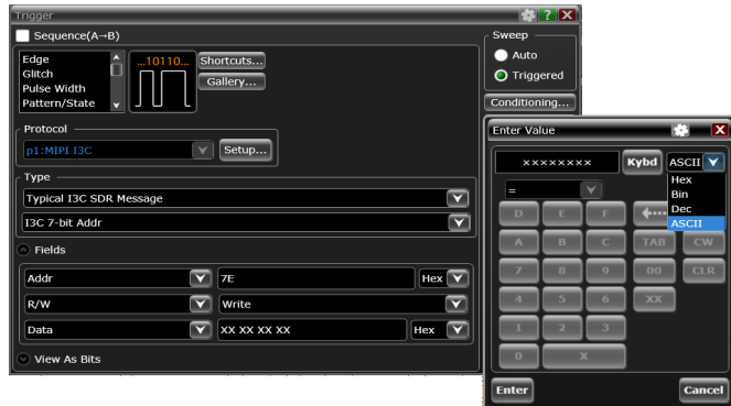
Figure 6. Using up to 3 field values of specific packet type, it is possible to trigger on specific pattern that you want to see.
