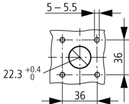
Diameter of drilled hole Door
