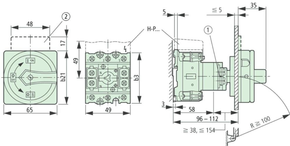
Shaft can be extended using ZVV-... + ZAV-..., max. F 4 × 25 = 100 mm
