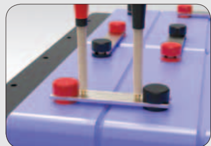
Safely measure the resistance of high voltage bus bars
