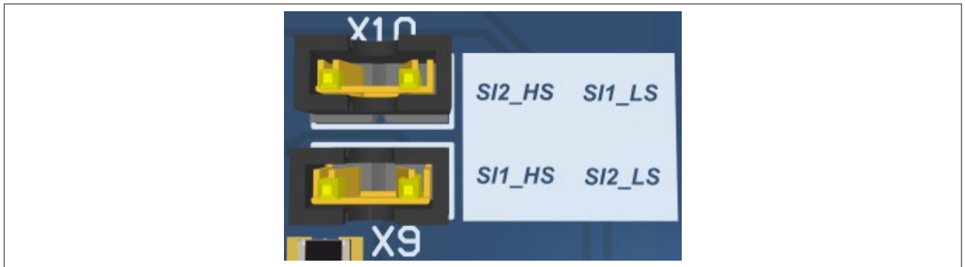
Figure 17 SI1, SI2 jumper cross-connect placement
