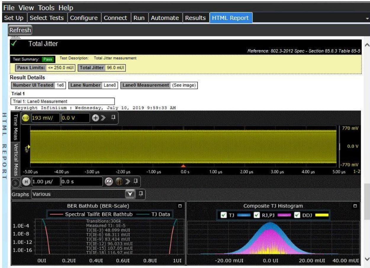
Figure 6. Additional details are available for each test, including the test limits, test description, and test results, including waveforms, if appropriate.
