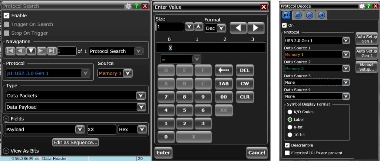
Figure 4. On the left is a comprehensive search system with a hex payload editor. On the right is the decode setup window.
