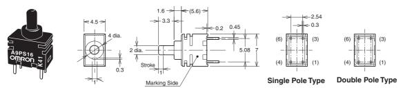
Note: NO.(4) and (6) terminals in the SPDT models are dummys to support the Switch case.
