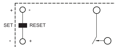
Wiring for L1 (Bottom View)
