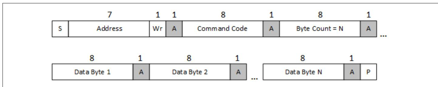
**Figure 24** Block Write
