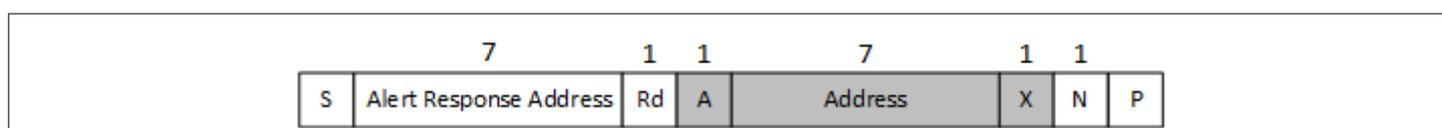
**Figure 30** A 7-bit-Addressable Device responds to an ARA
