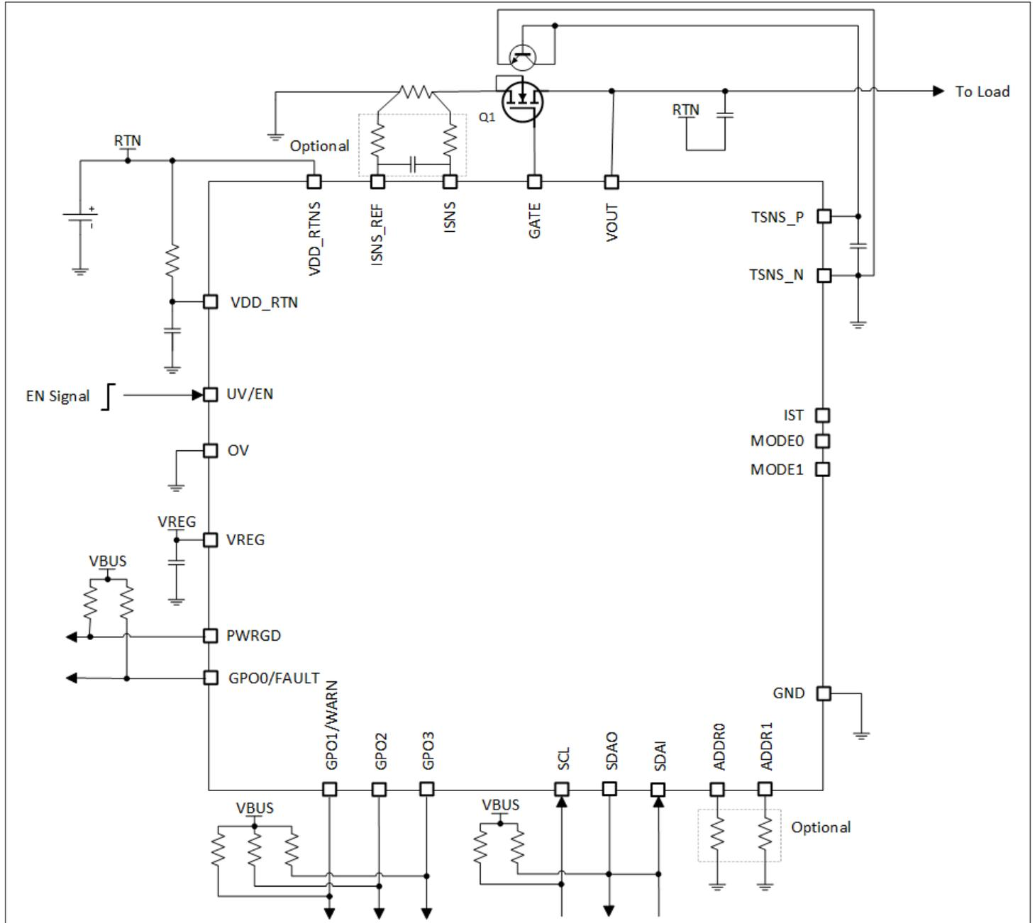
**Figure 32 Fully digital mode DCM (MODE:MODE=0x1) application schematic**
