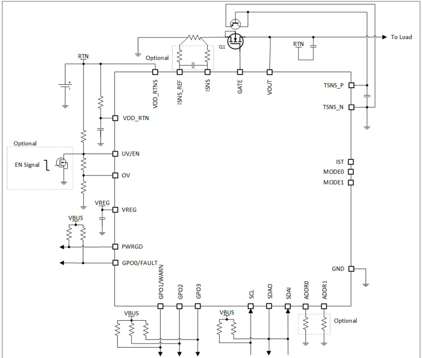
**Figure 33 Fully digital mode ACM (MODE:MODE=0x0) application schematic**
