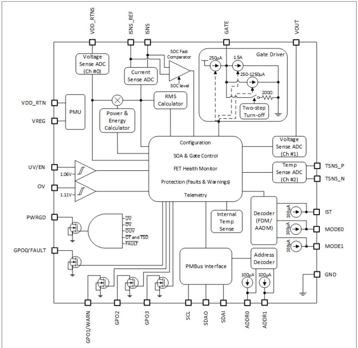
Figure 1 Block diagram
