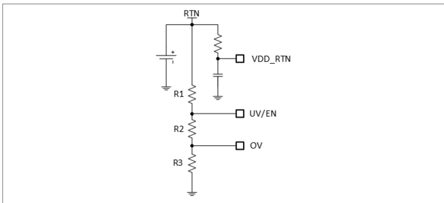
**Figure 35 Setting OV and UV in ACM**
