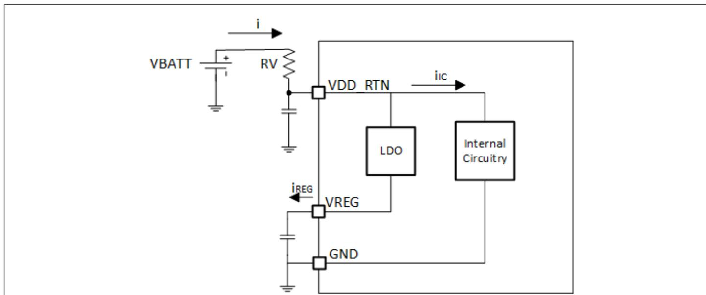
**Figure 36 Handling external current at VREG pin.**
