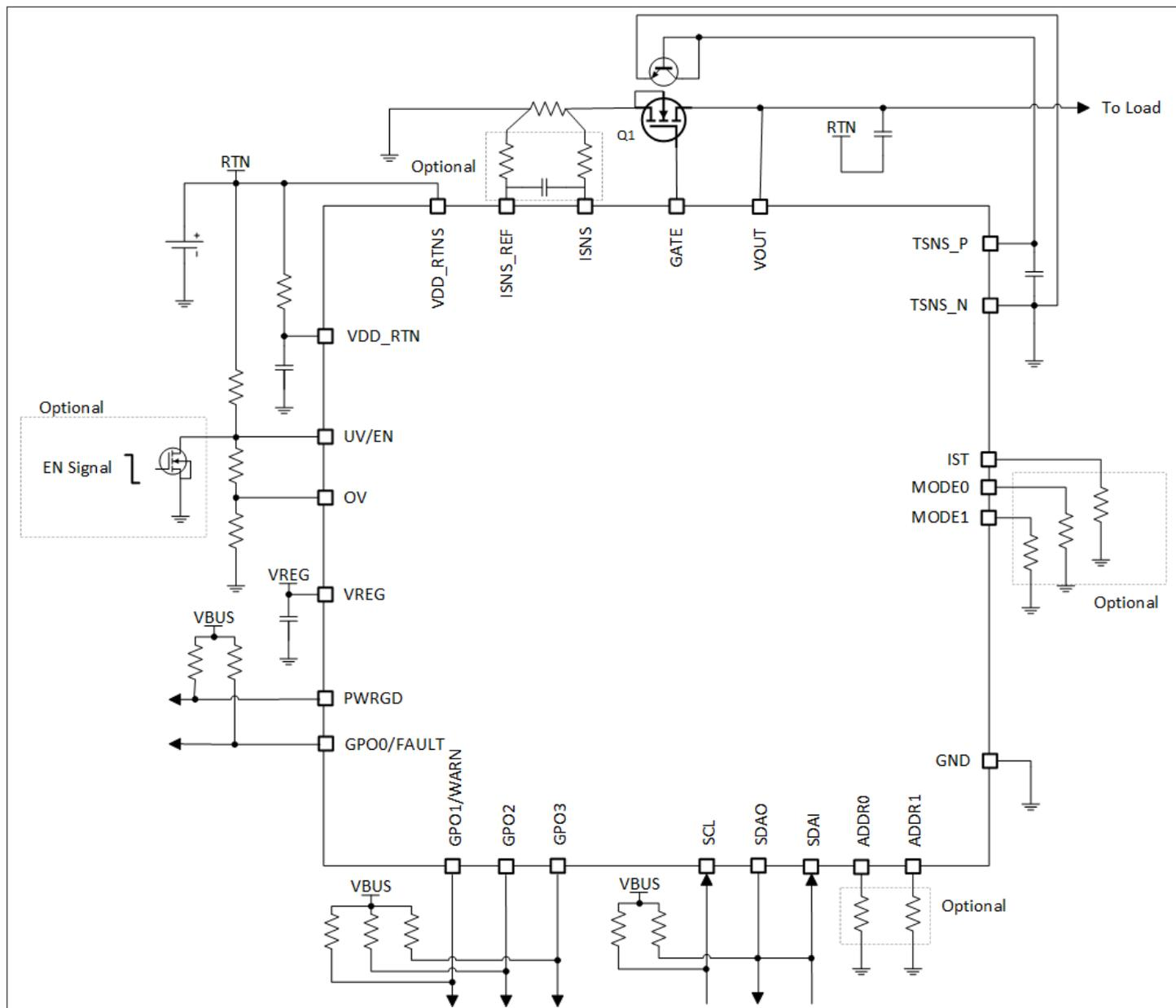
**Figure 34** Analog assisted digital mode application schematic
