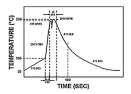
The Recommended solder Profile For Devices with Pb-free terminal plating used with leaded solder, or for devices with leaded terminal platingused with leaded
