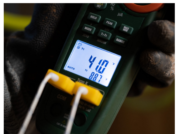
Dual Type K thermometer for taking differential temperature readings needed for superheat measurements.
