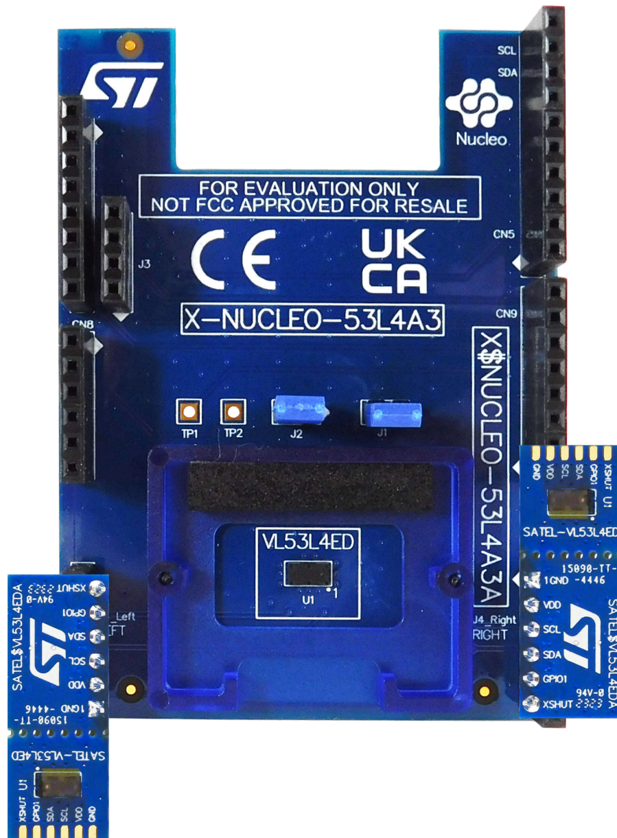
Figure 2. SATEL-VL53L4ED breakout boards connected to the X-NUCLEO-53L4A3 expansion board
