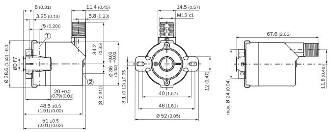
① Measuring point for operating temperature
