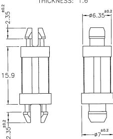
HOLE IN P.C.B: Ø4.8 THICKNESS: 1.6
