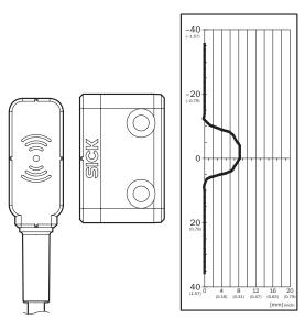
Safe switch on distance  $S_{\text{ao}}\,6~\text{mm}$
